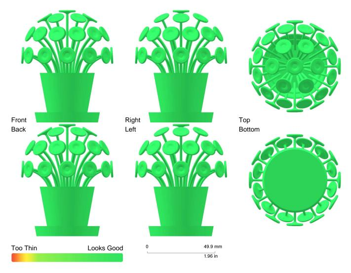
**Solidity Check** provides a heatmap of fragile areas (marked red) in your design. Despite these automatic checks, all designs go through a supplementary manual check, just to be sure.
