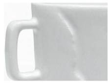
Ceramic is made by oven glazing after 3d-printing with a specific compound powder. The surface looks shiny and very smooth but weakly detailed. The objects are rigid, water and heat resistant.
