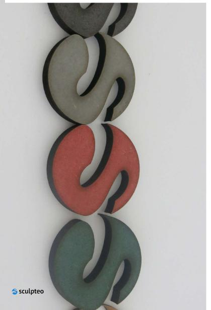
MDF stands for **Medium Density Fiberboard**. It is an engineered wood product made by breaking down hardwood or softwood residuals into wood fibres, combining it with wax and a resin binder, and forming panels. It is generally **denser than plywood** but can be used as a building material similar in application.
