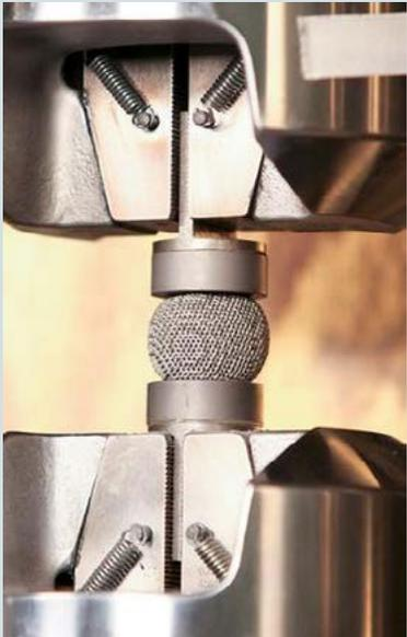
*Destructive test of titanium mesh sphere in lab at ORNL [2]*
