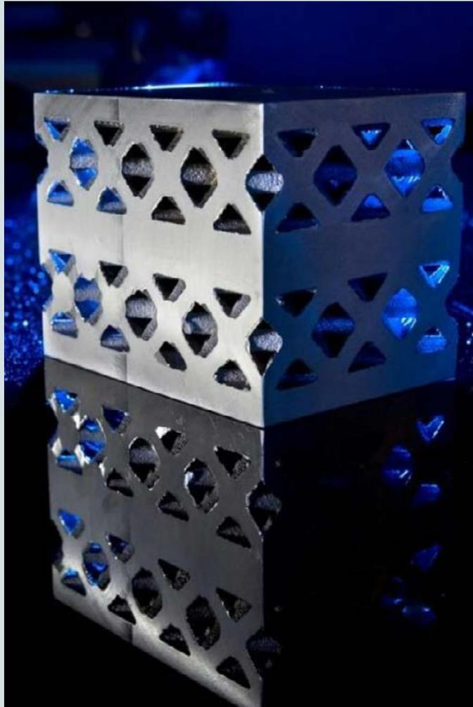
*The object shown here was created by using binder jetting technology to print the negative of this shape in casting sand. The casting sand model is then used to cast the complex geometry from aluminum in a typical foundry process.*
